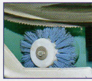
Chip removing wire brush assembly for longer Blade life
