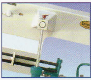
Adjustable cutting feed control valve
