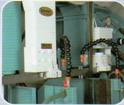
Roller Bearing / Carbide wear pad Blade Guide System
